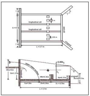
Fig.4. Design details of the proposed check dam on Kaju Nallah
