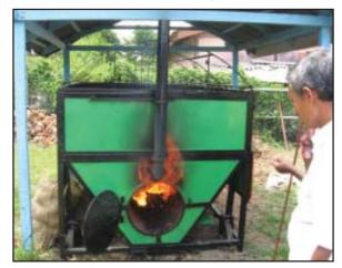
Plate 25. Biomass fired dryer
