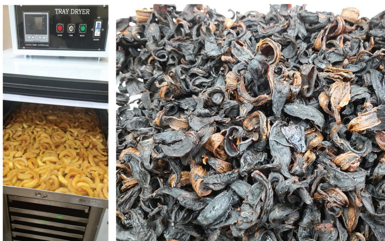
Mechanical drying of the rind (left) and produce after mechanical drying (right)
